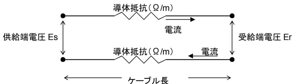
$E_s - E_r = \text{電圧降下}(V) = \text{ケーブル長} \times \text{導体抵抗} \times 2 \times \text{電流}$
