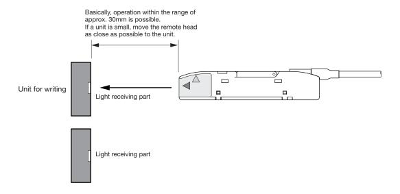
Basically, operation within the range of approx. 30mm is possible. If a unit is small, move the remote head as close as possible to the unit.
