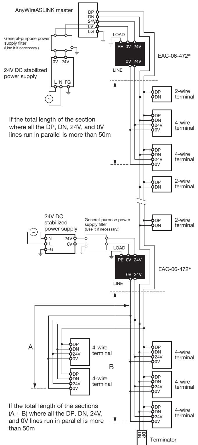
\* When using this filter, please be careful of the positions of LOAD and LINE.
