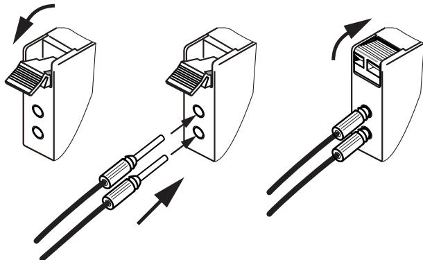
Attachment for fine fiber (E39-F9), manufactured by OMRON
