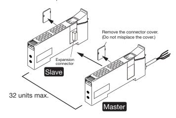
Up to 31 units of LB-F1011 can be connected to one unit of LA-F1011.
