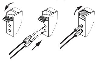
Attachment for fine fiber (E39-F9), manufactured by OMRON E39-F9 shall be separately purchased.
