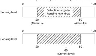
If this condition continues for 5000ms (equipment parameter 5:  $50 \times 100$ ms), it is detected as a drop in the sensing level and the user is notified with the ALM indicator on the unit and the alarm information is sent to the status detail area\*1 on the master unit.
