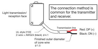
■Example of fitting the LP connector at the end of transmission line
