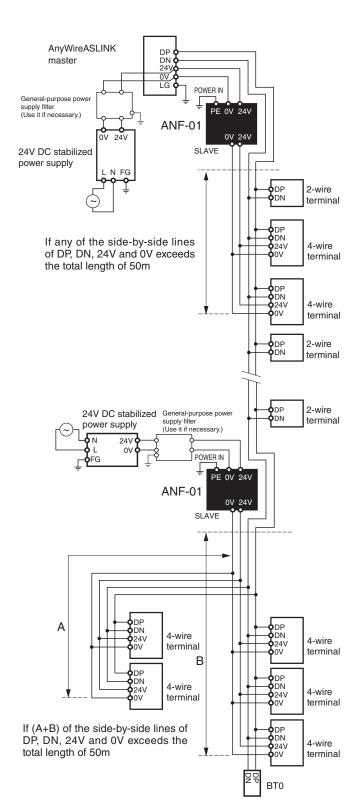
(The following is the explanatory connection diagram. Actual terminal arrangement should meet each device.)
