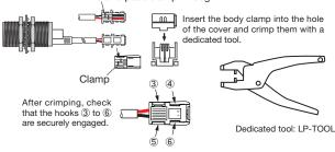
For the LP4-WW-10P, perform crimping with pin 1 for DN, pin 2 for DP, and pins 3 and 4 empty.
