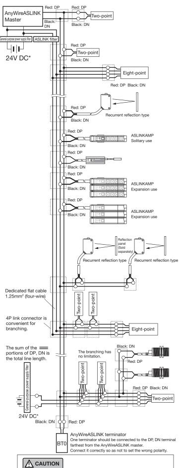
Make sure to use a four-wire (isolated) terminal if connecting to a load (e.g. input/output port) controlled by a different power supply than that used in the AnyWireASLINK. Otherwise, a malfunction may occur.
