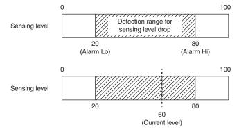
If this condition continues for 5000ms (equipment parameter 5:  $50 \times 100$ ms), it is detected as a drop in the sensing level and the user is notified with the ALM indicator on the unit and the alarm information is sent to the status detail area\* on the master unit.
