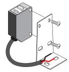
To secure the sensor, allow some extra length on the cable so that the cable and the connectors would not be subjected to any stress. Do not tighten the screws too tight. Doing so may cause a failure or a shift of light beam.
