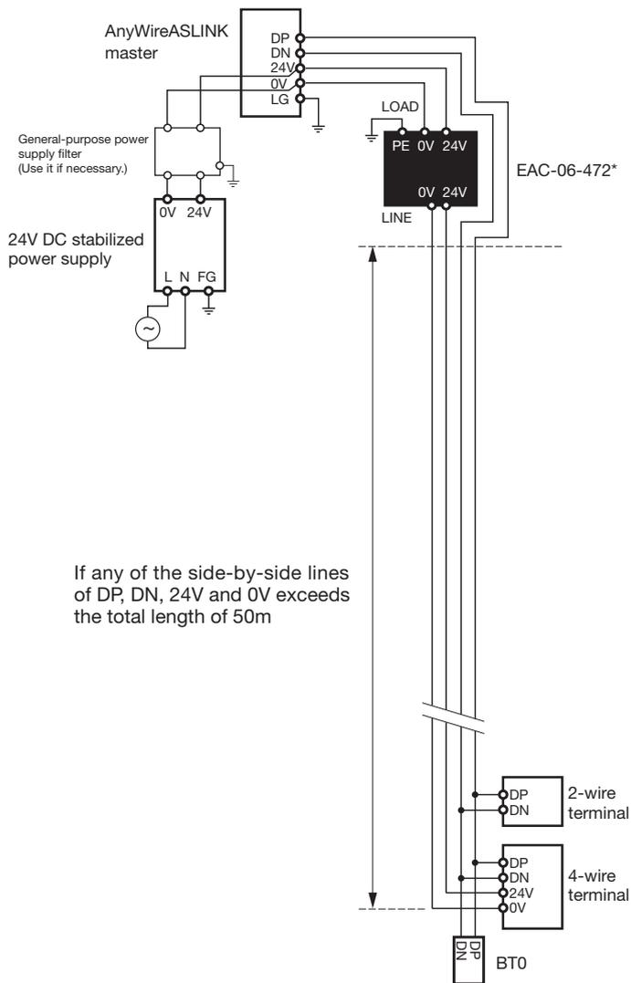
\* When using this filter, please be careful of the positions of LOAD and LINE.
