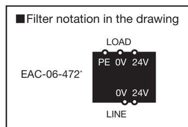
\* When using this filter, please be careful of the positions of LOAD and LINE.
