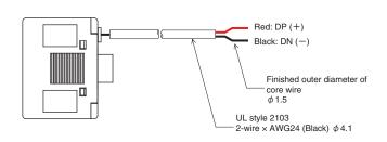
■ Example of fitting the LP connector at the end of transmission line connection cable
