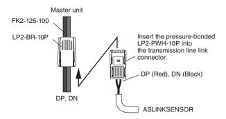
[When 4-pole LP connector (LP4-WW-10P) is used: Example of trunk cable with 2 wires]
