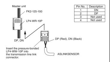
[When 4-pole LP connector (LP4-WW-10P) is used: Example of trunk cable with 4 wires]
