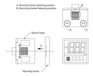
Insert the sensor body with the mounting frame into the panel hole, and put the mounting bracket from the back of the panel. Fix the mounting bracket with groove B while adjusting the mounting position.
