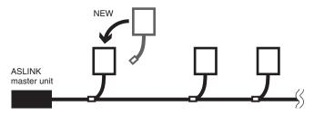
■ Step 4 Turn ON the 24V DC power supply for the master unit.
