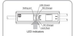
If an error is indicated, identify a cause of the error by checking lit/flashing status with the table on the left, and eliminate the cause of the error.
