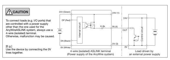
4-wire (isolated) NPN output BL296PB-16F-4A-20 BL296XB-16F-4A-20 (Output)
