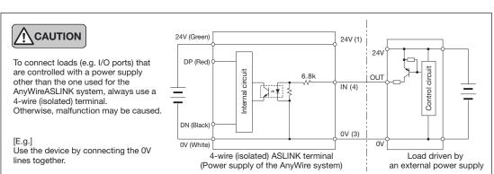
4-wire (isolated) PNP output BL296PB-16FS-4A-20 BL296XB-16FS-4A-20 (Output)
