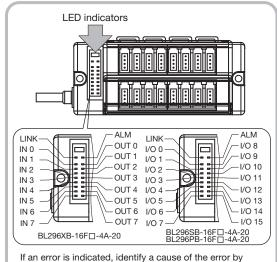
If an error is indicated, identify a cause of the error by checking lit/flashing status with the table on the left, and eliminate the cause of the error.
