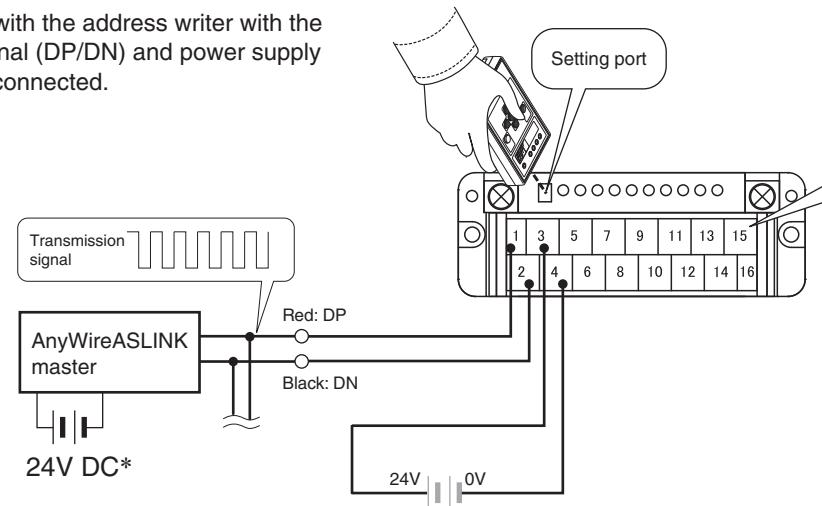
\* For the power supply to be connected, be sure to use a 24V DC stabilized power supply.
