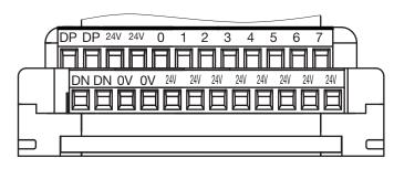
Terminals of the same symbol are internally connected with each other. 24V-0V total current: 0.8A max.
