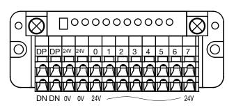
Terminals of the same symbol are internally connected with each other. 24V-0V total current: 0.8A max.
