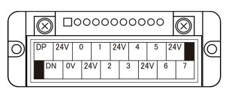
Terminals of the same symbol are internally connected with each other. 24V-0V total current: 0.8A max.
