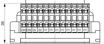
\* This figure shows an example of terminal layout of the NPN 8-point output type.
