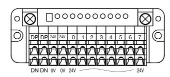
Terminals of the same symbol are internally connected with each other. 24V-0V total current: 0.8A max.
