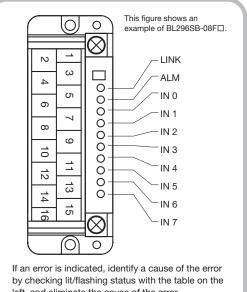
left, and eliminate the cause of the error. Once the cause of the error is eliminated, the error indication will be automatically reset.
