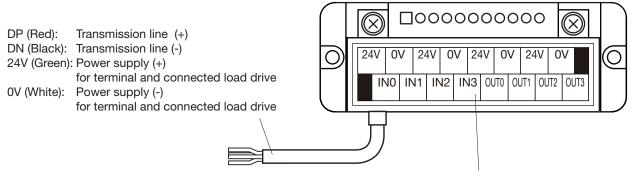
The 24V terminal of the transmission line connection cable is internally connected to the 24V pin of the terminal block. The 0V terminal of the transmission line connection cable is internally connected to the 0V pin of the terminal block. Terminals of the same symbol are internally connected with each other.
