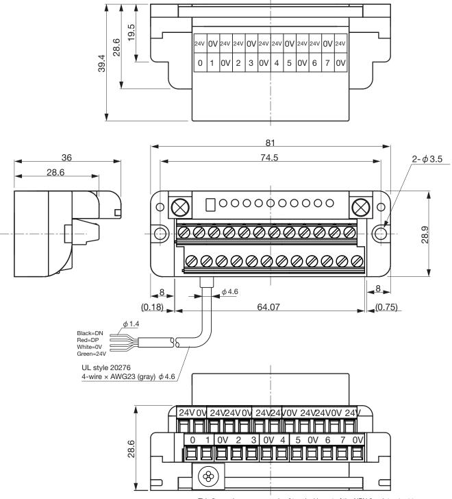
\* This figure shows an example of terminal layout of the NPN 8-point output type.
