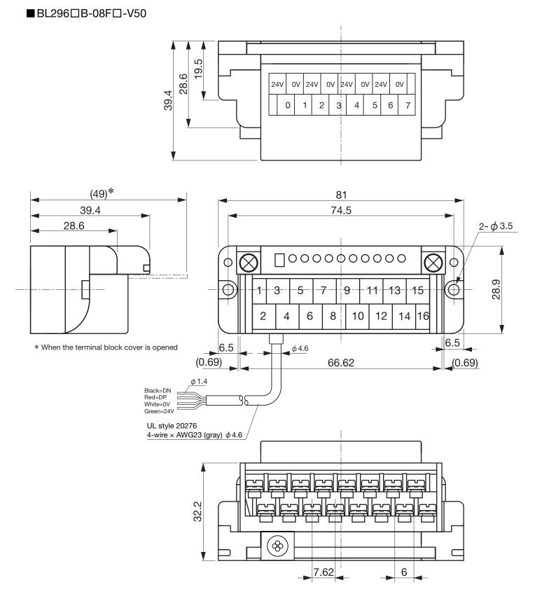
M3, 6.42mm pitch, compatible with crimp terminal of 6mm in width
