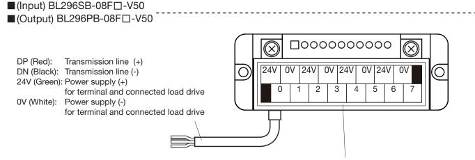
The 24V terminal of the transmission line connection cable is internally connected to the 24V pin of the terminal block. The 0V terminal of the transmission line connection cable is internally connected to the 0V pin of the terminal block. Terminals of the same symbol are internally connected with each other.
