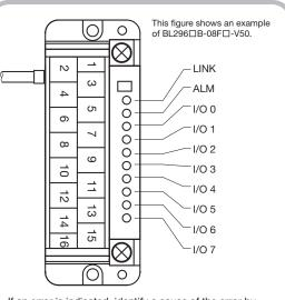
If an error is indicated, identify a cause of the error by checking lit/flashing status with the table on the left, and eliminate the cause of the error. Once the cause of the error is eliminated, the error indication will be automatically reset.
