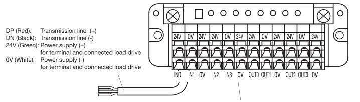
The 24V terminal of the transmission line connection cable is internally connected to the 24V pin of the terminal block. The 0V terminal of the transmission line connection cable is internally connected to the 0V pin of the terminal block. Terminals of the same symbol are internally connected with each other.
