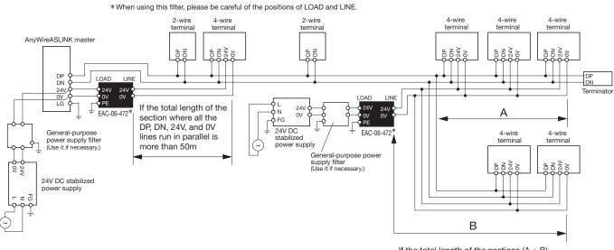
If the total length of the sections (A + B) where all the DP, DN, 24V, and 0V lines run in parallel is more than 50m
