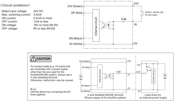
4-wire (isolated) PNP output BL296PB-08FS-00-V50 BL296XB-08FS-00-V50 (Output)
