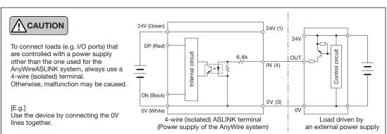
4-wire (isolated) PNP output BL296PB-08FS-4A-20 BL296XB-08FS-4A-20 (Output)
