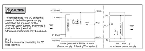
4-wire (isolated) NPN output BL296PB-08F-4A-20 BL296XB-08F-4A-20 (Output)
