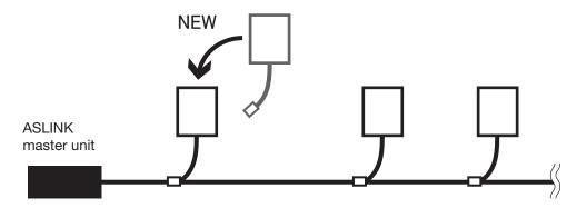
■ Step 4 Turn ON the 24V DC power supply to the master unit.
