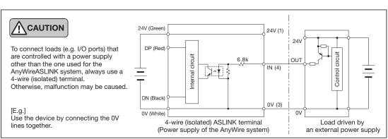
4-wire (isolated) PNP output BL296PB-08FS-4A-20 BL296XB-08FS-4A-20 (Output)
