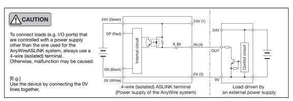
4-wire (isolated) NPN output BL296PB-08F-4A-20 BL296XB-08F-4A-20 (Output)
