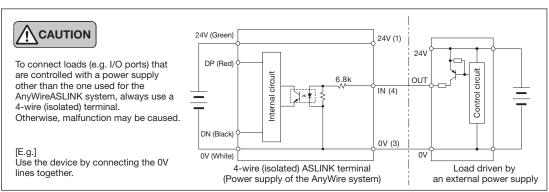
4-wire (isolated) PNP output BL296PB-08FS-4-20 BL296XB-08FS-4-20 (Output)
