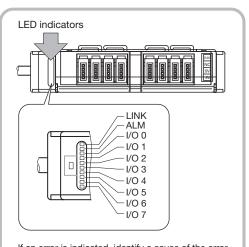
If an error is indicated, identify a cause of the error by checking lit/flashing status with the table on the left, and eliminate the cause of the error. Once the cause of the error is eliminated, the error indication will be automatically reset.
