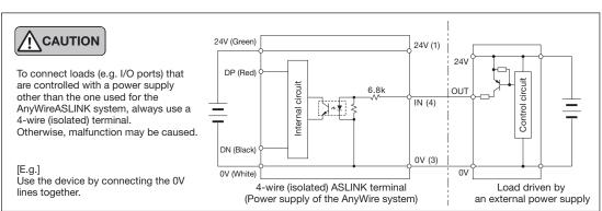
4-wire (isolated) PNP output BL296PB-08FS-4-20 BL296XB-08FS-4-20 (Output)
