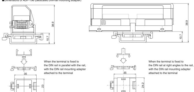
\*The above figures show examples of the terminal with e-CON socket (BL296 -08-4). The same dimensions apply to the models with JST connector (BL296 -08-9) and Molex connector (BL296 -08-10).
