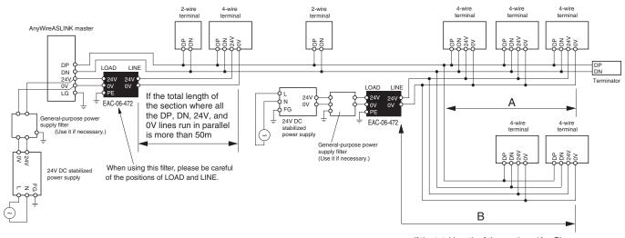
If the total length of the sections (A + B) where all the DP, DN, 24V, and 0V lines run in parallel is more than 50m
