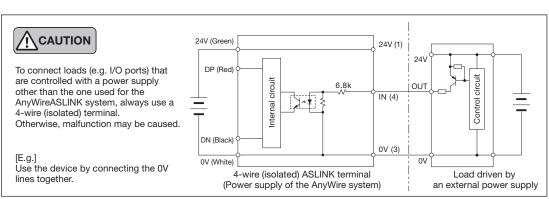
4-wire (isolated) PNP output BL296PB-04FS-4A-20 BL296XB-04FS-4A-20 (Output)
