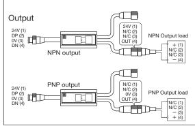
To connect loads (e.g. I/O ports) that are controlled with a power supply other than the one used for the AnyWireASLINK system, always use a 4-wire (isolated) terminal.
