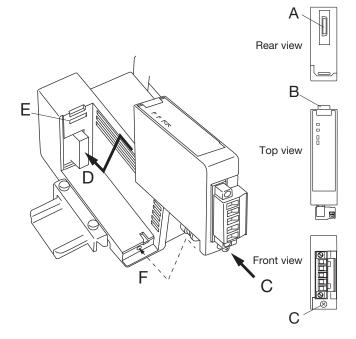
This manifold driver is intended for the MN4G-T70-FL series manifold manufactured by CKD Corporation. Mount the driver to the specified manifold. (Purchase the manifold separately.) MN4G-T70-FL can be connected to a solenoid valve quickly with the plug-in connector.
