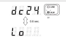
If the voltage of 24V DC power supplied to the unit becomes significantly low (near 16V), the message "dc24 Lo" is displayed and the unit stops functioning. Check the supply voltage and take actions to increase the voltage to the allowable range.
