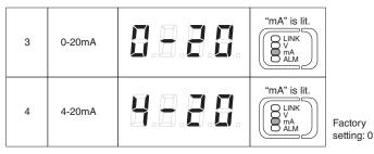
After startup at receipt of a transmission signal, the preset input specification setting is displayed for approx. 3 seconds, and then the display changes to indicate an actual input value.
