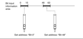
In the case where the unit is used with word address setting
