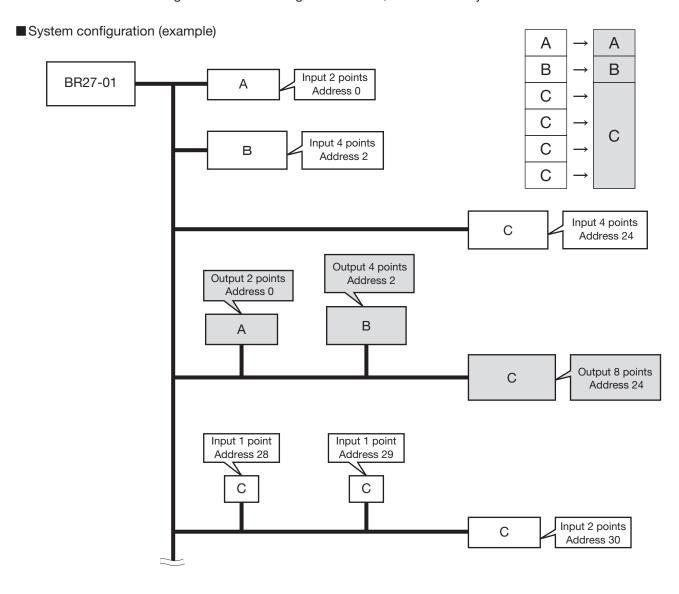
■ Input signals and corresponding output signals
