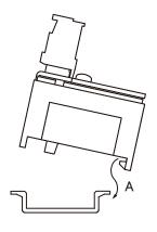
Lower the B side of the hook, and engage the DIN rail with the slide hook C.
