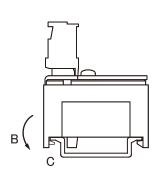
To remove the unit, pull the slide hook C outward. After raising the unit body in the direction of D, remove the fixed hook A from the DIN rail.
