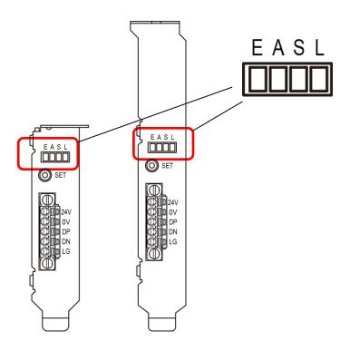
The LEDs are labeled as "E", "A", "S", and "L", and each one can be used to indicate in either "Normal mode" or "Board ID display mode."
