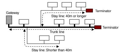
When the system has a stay line of 40m or longer
