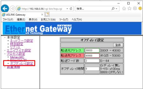
For transfer destination address, Modbus/TCP memory addresses 49745 to 50000 (User available area) can be used.
