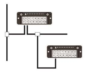
Actual wiring will be the same as the T-branching method or multi-drop method.
