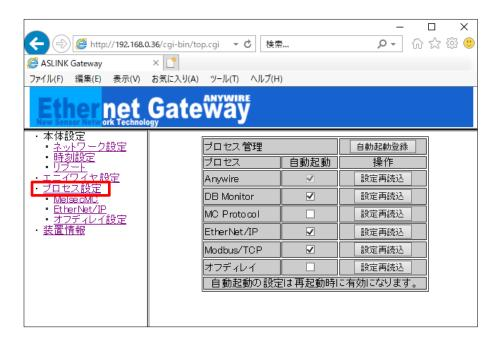
The number of points setting in the AnyWireASLINK system, SLMP (MC protocol) setting and EtherNet IP setting can be reflected from this screen.
