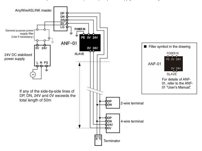
■ Connection example of ASLINK filter (ANF-01) for local power supply
