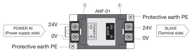
\*The PE terminal is internally connected.
