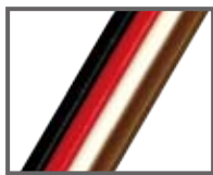
4芯扁平电缆 AWG16 (1.25sq) × 4芯 (从左起DN:DP:0V:24V)
