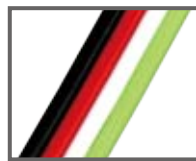
4芯扁平电缆 AWG18 (0.75sq) × 4芯 (从左起DN:DP:0V:24V)
